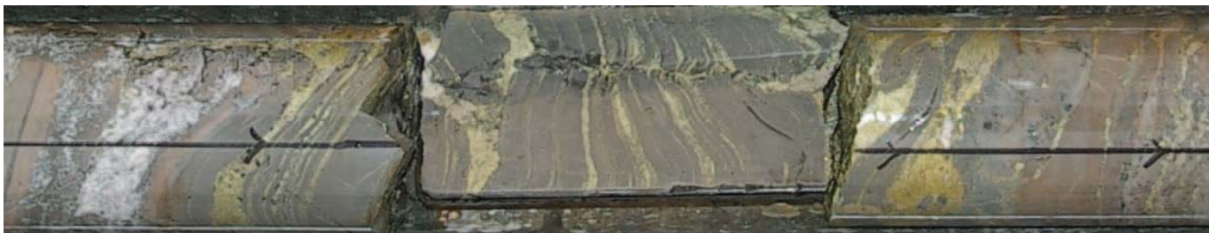
FIG 5 – Vein and associated bedding plane replacement-style chalcopyrite mineralisation emanating from a biotite ± carbonate vein in hard grey albitite from Havilah drill hole KKDD0286, 212.8 m.
