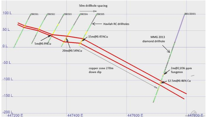
Havilah drillholes CRRC 1 to 5 were all sited to intersect the interpreted copper mineralised horizon (defined by the red lines) that was projected some 300-400 metres up-dip from the earlier MMG diamond drillhole BNG13DDO01.
