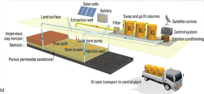
Swap and go ion-exchange resin columns will allow development of a spoke and hub development concept over far-flung sand-hosted uranium deposits
